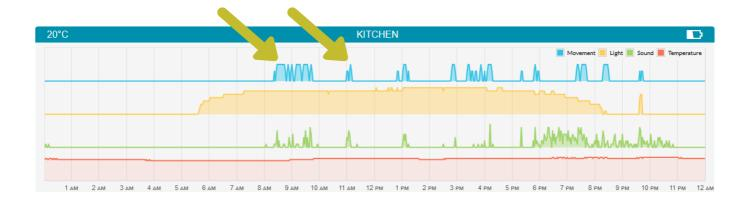
Placing a door sensor on the fridge can also indicate that they are eating and drinking. Door sensor movement is shown as blue line bars on the corresponding door sensor graph.
