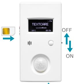
Switch on the Main Sensor by sliding the ON/OFF switch, located on its right-hand side.
